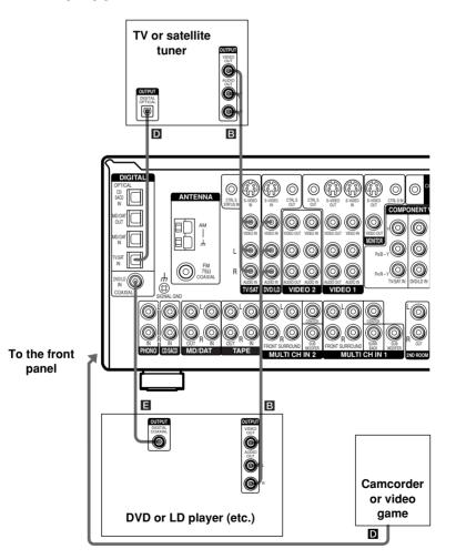
WW Connect the digital output jacks of your MD or DAT deck to the receiver's digital input jack and connect the digital input jacks of your MD or DAT deck to the receiver's digital output jack. These connections allow you to make digital recordings of TV broadcasts, etc.
