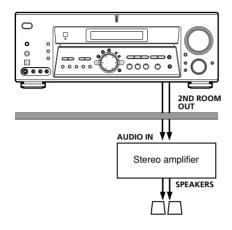
Press 2ND ROOM repeatedly to select the analog audio signals for output to a stereo amplifier in another room. For details on the connection, see page 15.
